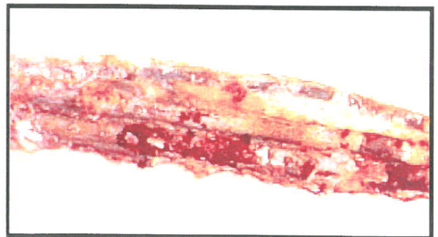
CLOSE UP (25X) OF UNPROTECTED AREA SHOWING PITTING, METAL LOSS AND SEVERE CORROSION (1000 HRS SALT SPRAY EXPOSURE)
